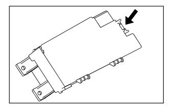
To access the fuse block, pull out and lift up on the cover latch, located at the end of the fuse block, near the battery cable.
